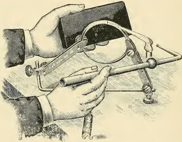
thereby concentrating the heat, the same as when held directly upon it. In soft soldering it can be used to great advantage.
