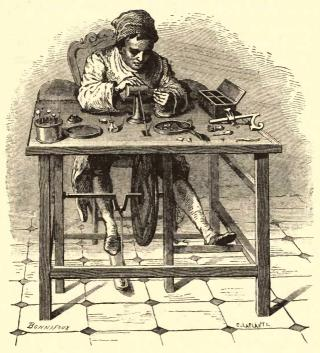
Fig. 123.—The Lathe at work.
