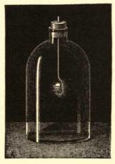
Fig. 33.—Combustion of the Diamond in Oxygen.
