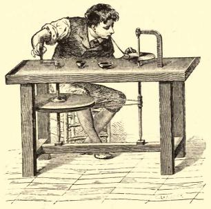
Fig. 125.—Apparatus for Sawing Hard Stones.
