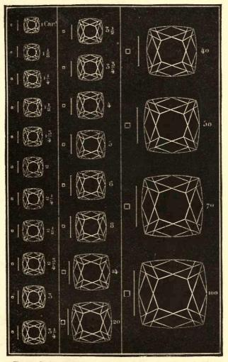
Fig. 5t.+Surfaces of Brilliants compared to their weight. The vertical lines indicate the thickness of the stone.
